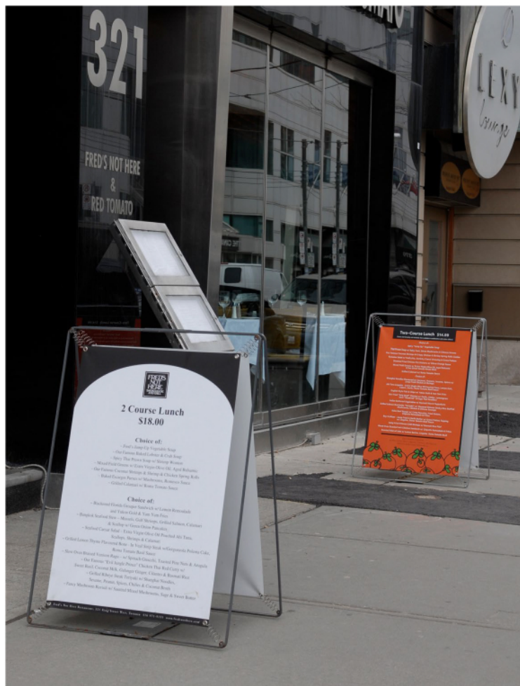
The center pad folds down and provides a platform to weigh the display down for wind resistance. It can also be cabled for extra security.
